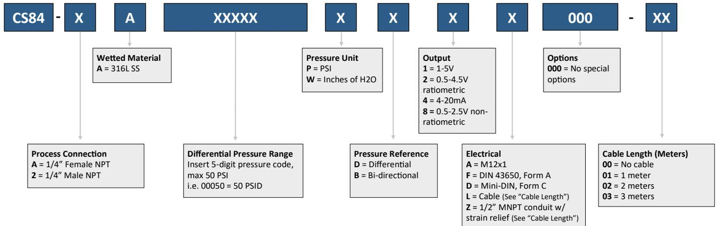
**Ordering Example:** CS84-AA00010PD4A000-00 (1/4" Female NPT, 316L SS, 0-10 PSI differential, 4-20mA, M12x1)
