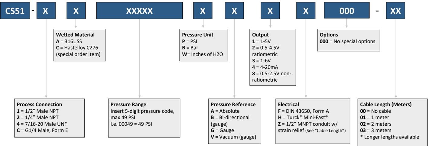
**Ordering Example:** CS51-2A00010PG4H000-00 (1/4" Male NPT, 316L SS, 0-10 PSI gauge, 4-20mA, Turck® Mini-Fast®)
