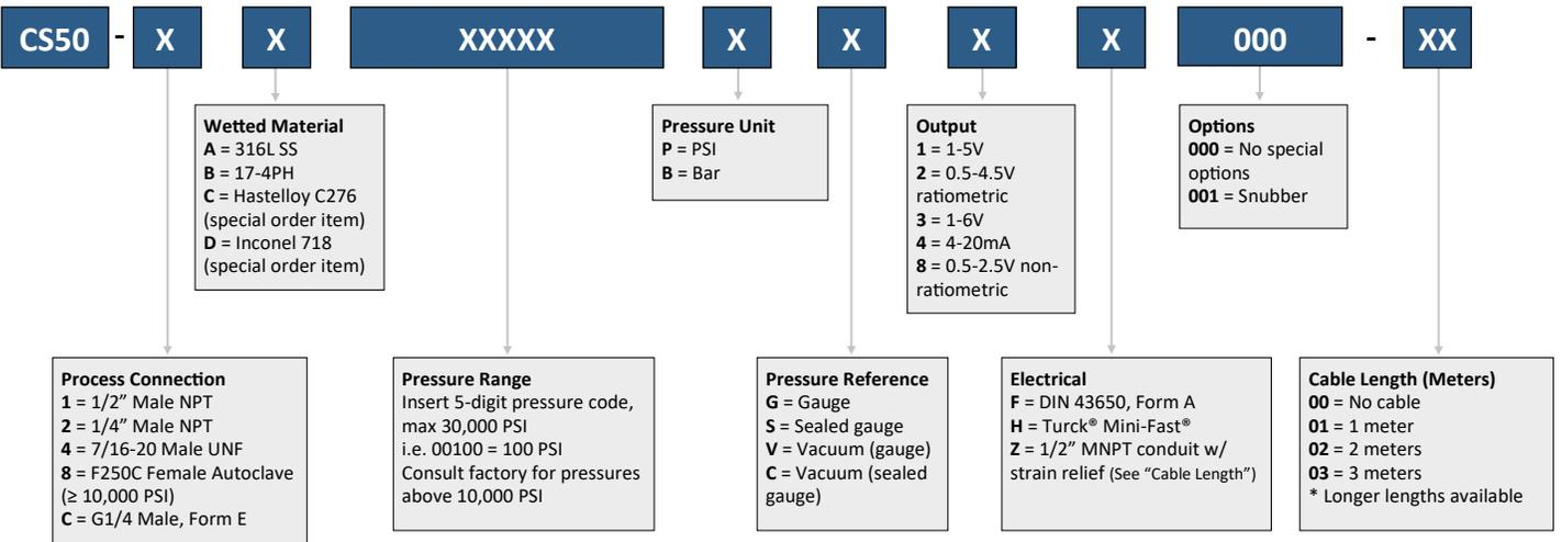
**Ordering Example:** CS50-1A00200PG4H000-00 (1/2" Male NPT, 316L SS, 0-200 PSI gauge, 4-20mA, Turck® Mini-Fast®)
