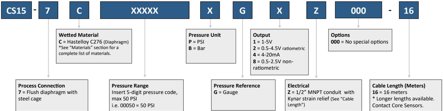
**Ordering Example:** CS15-7C00010PG4Z000-16 (Steel cage, Hastelloy C276, 0-10 PSI gauge, 4-20mA, 1/2" MNPT conduit w/ Kynar strain relief, 16 meter cable)
