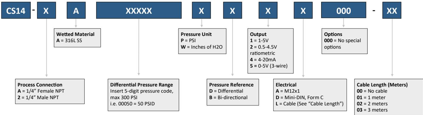
**Ordering Example:** CS14-AA00010PD4A000-00 (1/4" Female NPT, 316L SS, 0-10 PSI differential, 4-20mA, M12x1)
